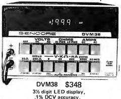
3½ digit LED display, .1% DCV accuracy, AC operated, auto-ranging, auto-zero, king size pushbuttons
